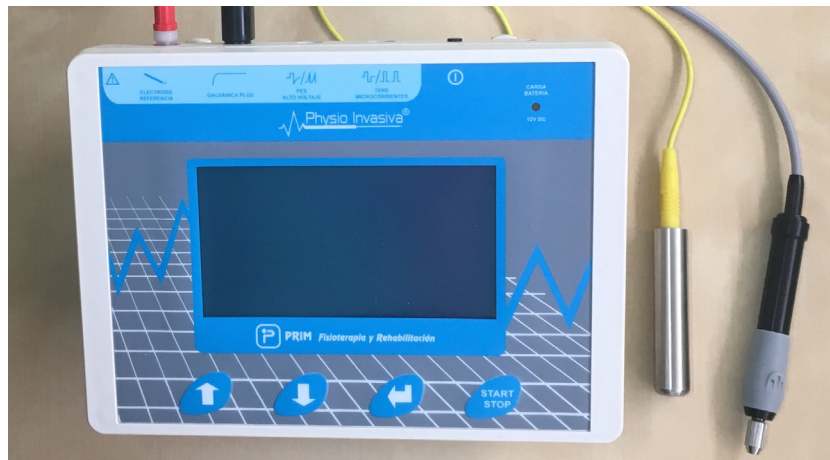
Fig. 1. PNE unit employed in this trial. The device generates a galvanic current that is transferred to the target structure through acupuncture-like needles.
